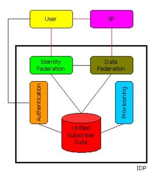
Figure 5.3-a: Reference architecture for identity management.
